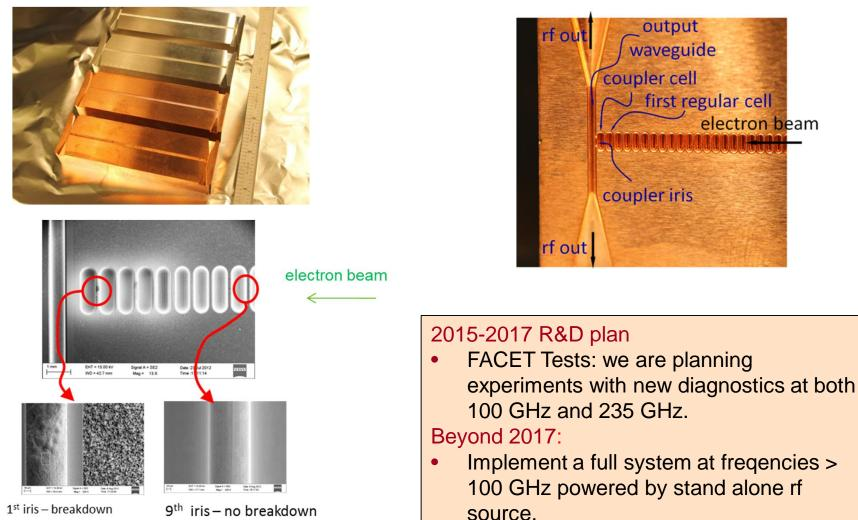
1<sup>st</sup> iris – breakdown damage, peak surface fields ~0.5 GV/m 9<sup>th</sup> iris – no breakdown damage, peak surface fields > 0.2 GV/m, pulse length ~3ns
