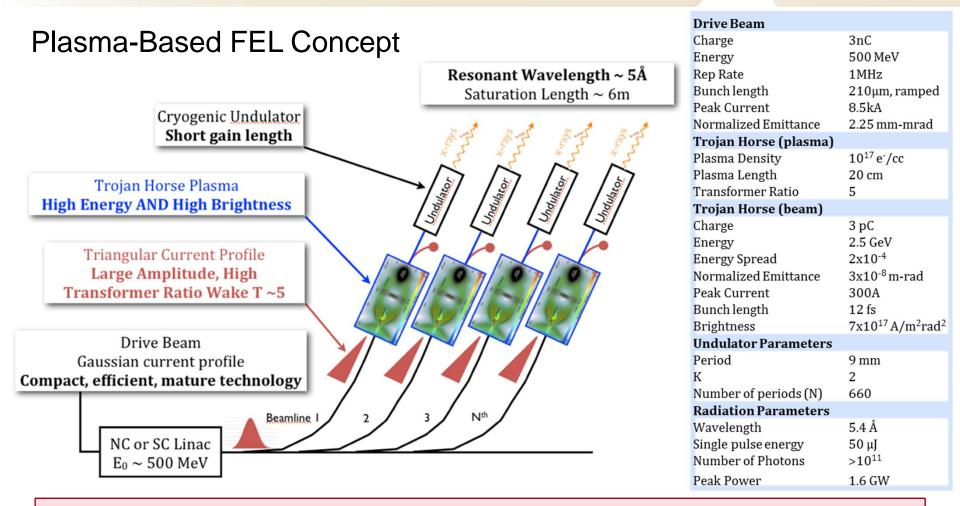
Leverage high rep-rate beam drivers with plasma as source of highbrightness high-energy electrons
