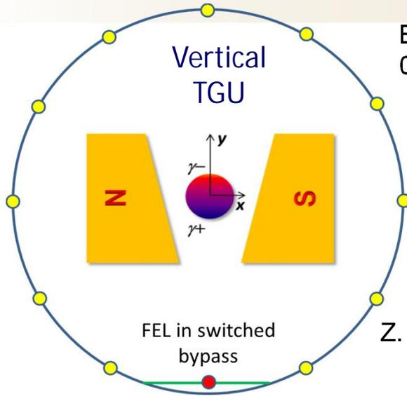
$E = 4.5 \text{ GeV}$   $\varepsilon_{x/y} = 160 / 1.6 \text{ pm}$   $\delta E/E = 1.6 \times 10^{-3} \text{ rms}$   $Q = 0.75 \text{ nC}$   $\eta_y = 0.05 \text{ m}$   $\beta_{x/y} = 16 / 50 \text{ m}$   $\sigma_\beta = 52 \text{ mm}$   $\sigma_\eta = 78 \text{ mm}$   $\lambda_u = 3 \text{ cm}$   $K = 3.7$
