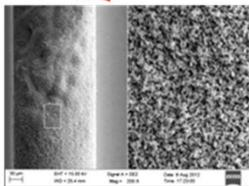
1<sup>st</sup> iris – breakdown damage, peak surface fields  $\sim 0.5$  GV/m
