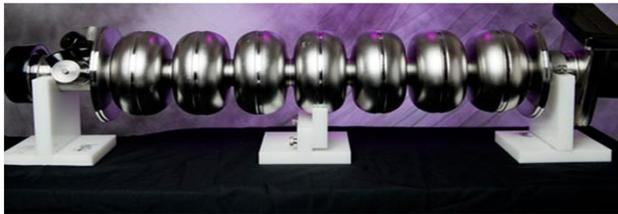
8 CEBAF SC cavities in a cryomodule produce 108 MV for longitudinal focusing
