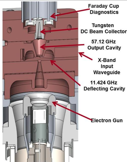
V-band Device uses over-moded cavities for high frequency generation (57.12 GHz)
