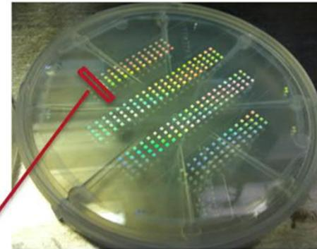
bonded silica phase reset accelerator prototypes fabricated at SLAC/Stanford
