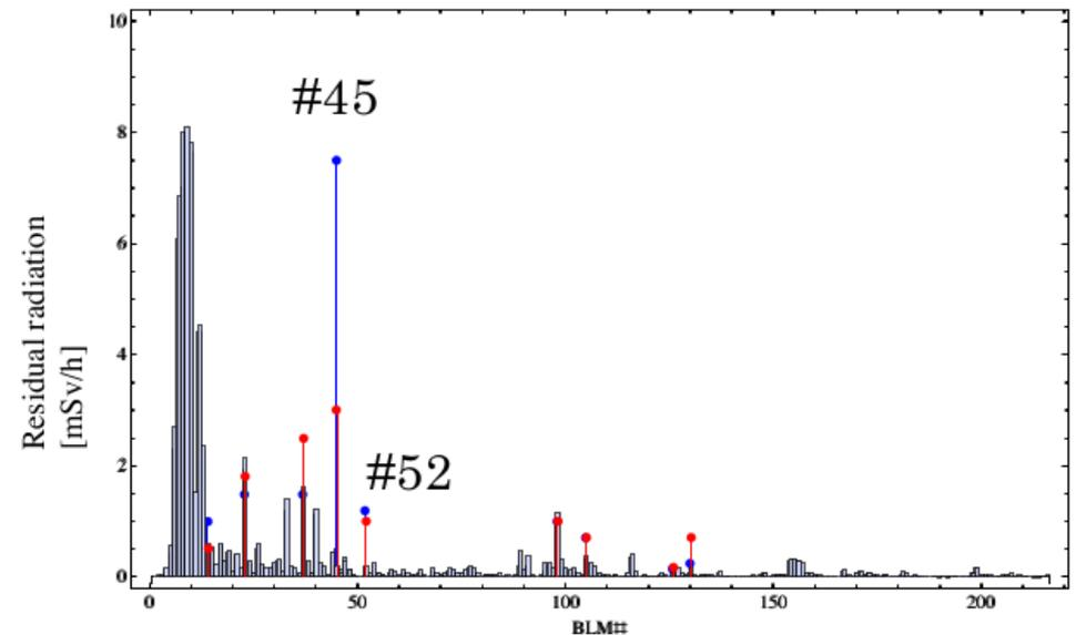
Figure 1: Beam loss signals during operation vs. residual radiation measured with the BLMs.
