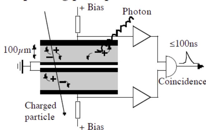
*The charged particle crosses both PIN-diodes, causing a coincidence. Synchrotron radiation photons, if stopped by either PIN-diode, do not cause a coincidence*
