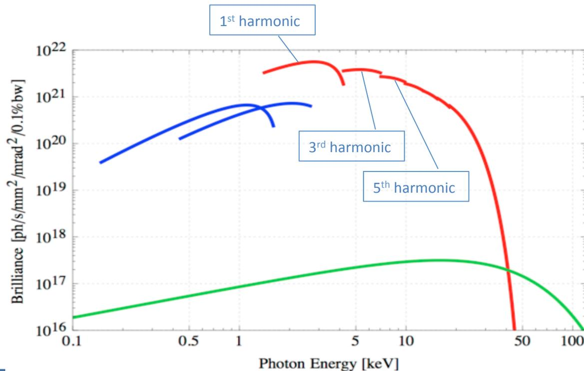
Red curve: tuning range for Sirius IVU19 undulator.  $\lambda_u=19$  mm, minimum gap=4.5 mm ( $K=2.3$ )
