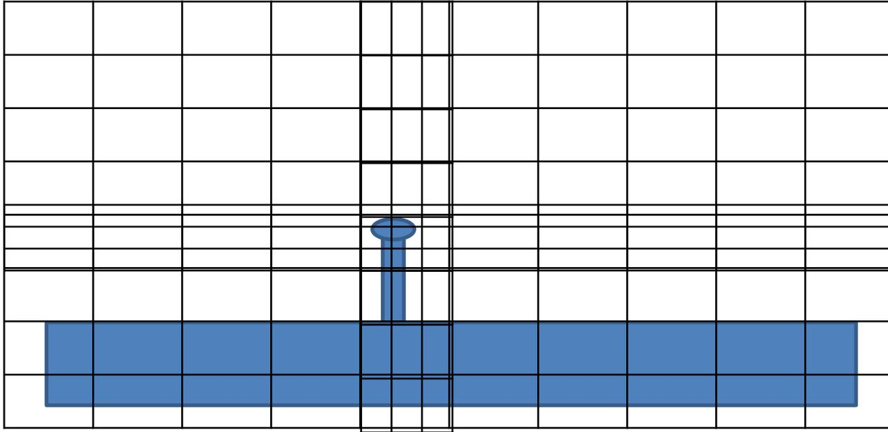
One drawback of a conformal mesh is you cannot refine the mesh at critical points without refining the mesh along a cross pattern in all directions.
