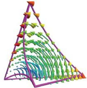
The domain is then discretized into curved tetrahedral elements and  $\int E d\tau$  is represented as an expansion in hierarchical Whitney vector basis functions  $N_i(\mathbf{x})$
