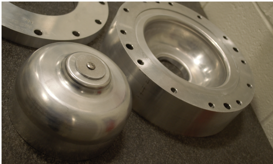
Figure: Dice for half cell elliptical cavity deep pressing.
