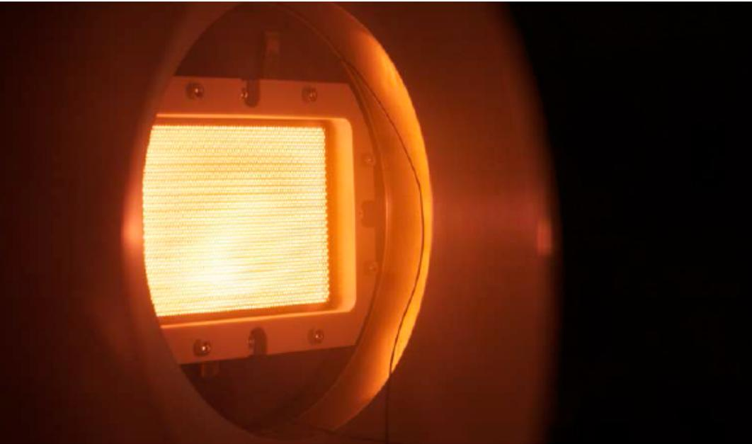
The electronic propulsion is more efficient, but space charge limit the power
