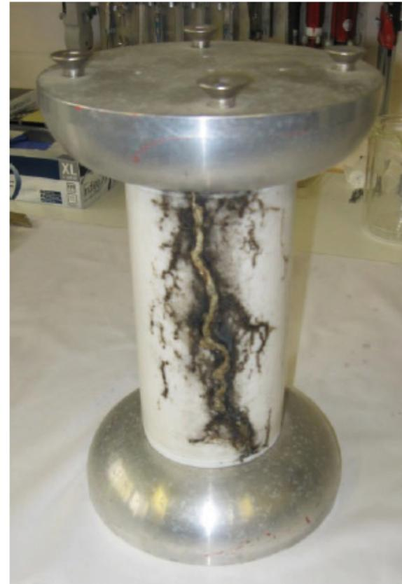
Breakdown by water leak
