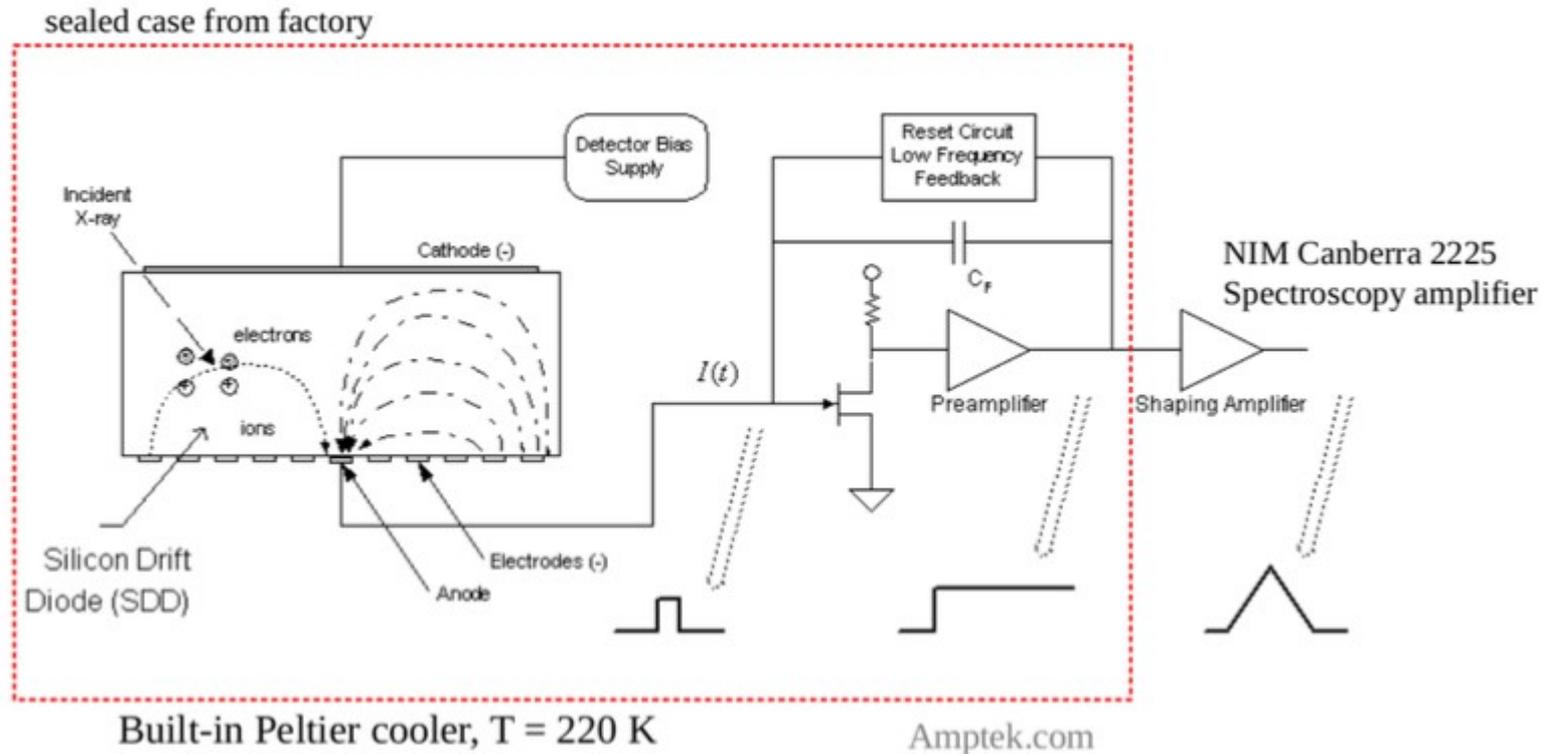
We used an X-ray detector which is a Silicon Drift Diode, 29mg mass
