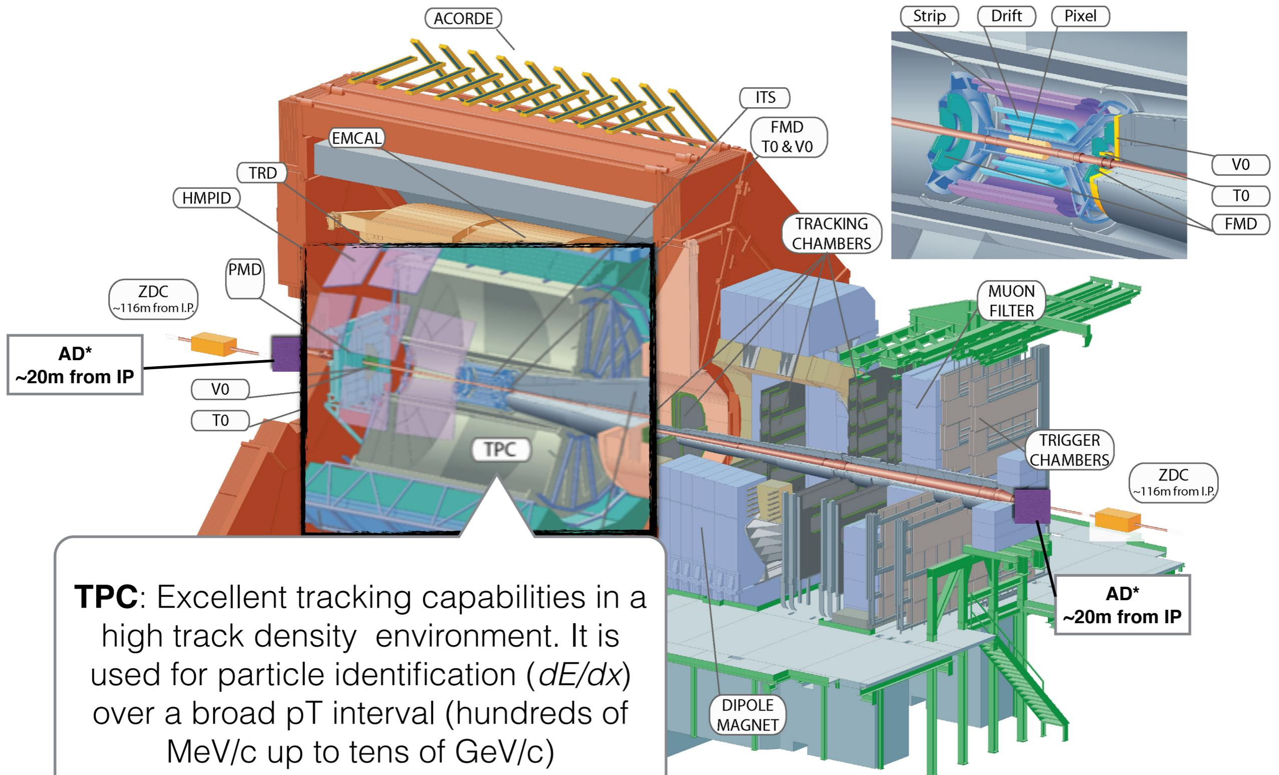
**TPC:** Excellent tracking capabilities in a high track density environment. It is used for particle identification ( $dE/dx$ ) over a broad  $p_T$  interval (hundreds of MeV/c up to tens of GeV/c)
