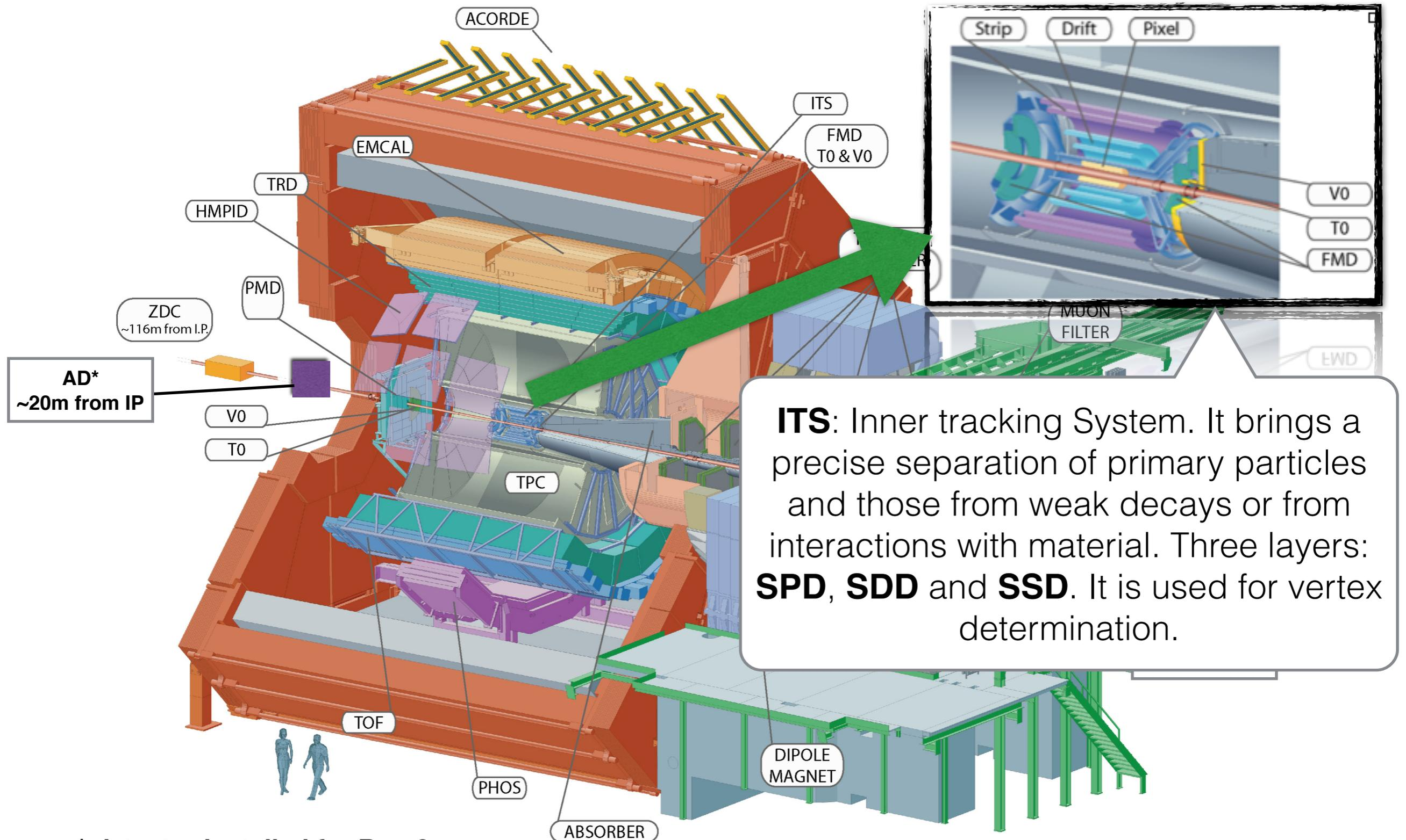
**ITS:** Inner tracking System. It brings a precise separation of primary particles and those from weak decays or from interactions with material. Three layers: **SPD**, **SDD** and **SSD**. It is used for vertex determination.
