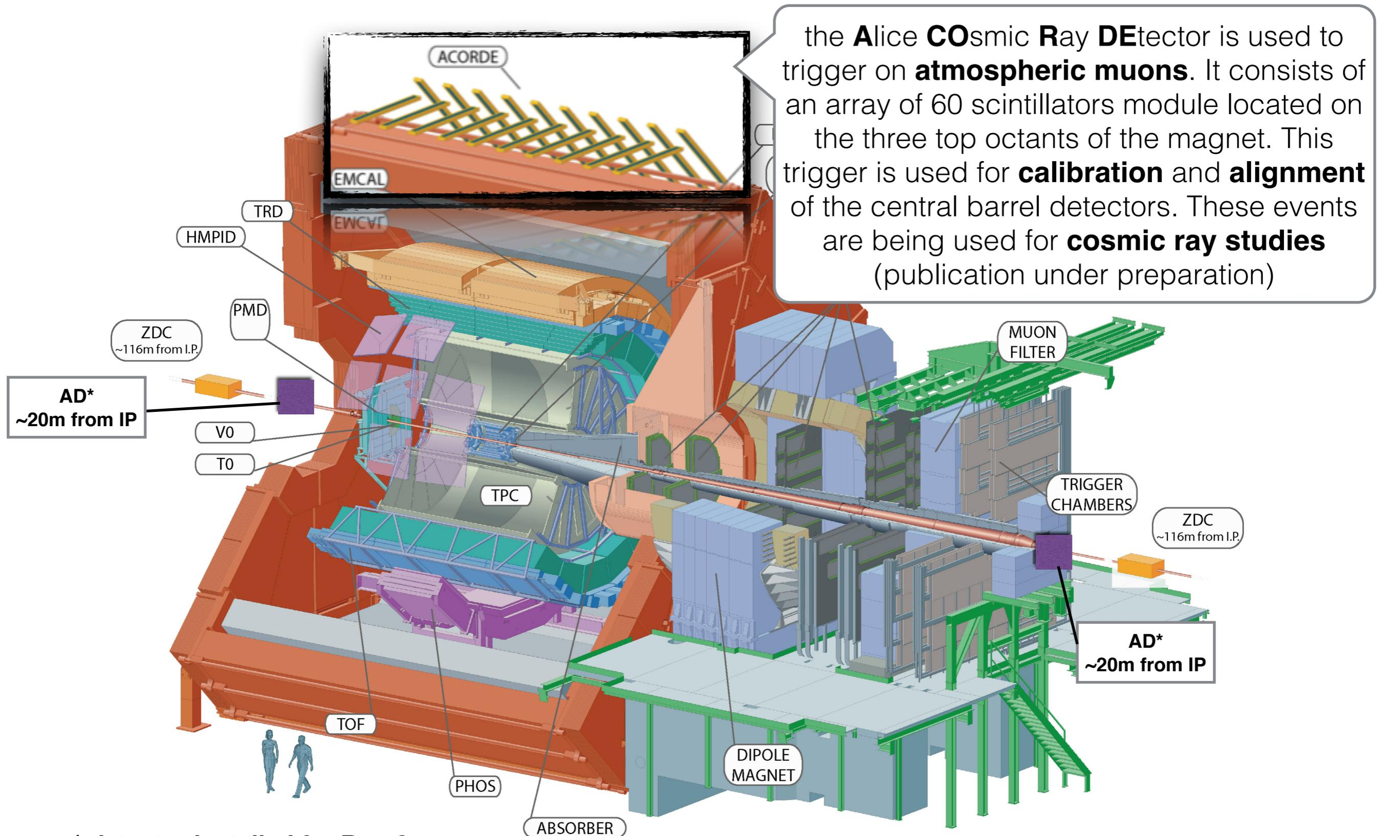
the **Alice COsmic Ray DEtector** is used to trigger on **atmospheric muons**. It consists of an array of 60 scintillators module located on the three top octants of the magnet. This trigger is used for **calibration** and **alignment** of the central barrel detectors. These events are being used for **cosmic ray studies** (publication under preparation)
