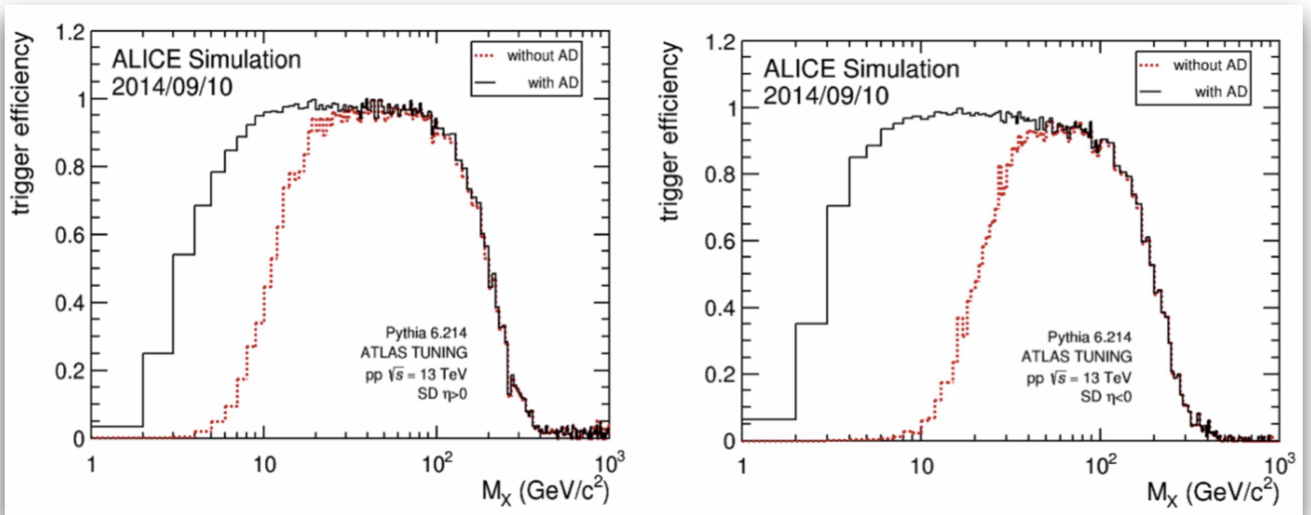
The AD detector will increase the sensitivity to diffractive masses close to threshold ( $m_\rho + m_\pi$ ) and also partially compensate for the loss of trigger efficiency for MB events
