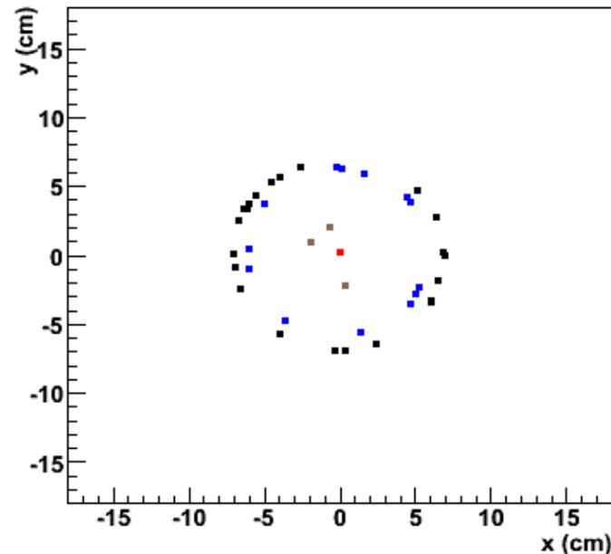
Photon hit position on the CsI photocathode. The rings are from one event of one incident 16 GeV/c pion (black), one kaon (blue) and one proton (brown).
