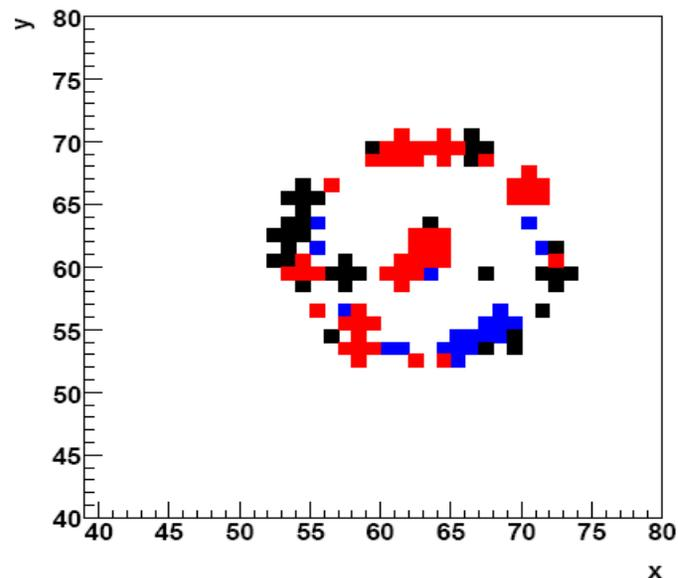
Ring image detected on MWPC. The rings are from one event of one incident  $16 \text{ GeV}/c$  pion (black), one kaon (blue) and one proton (red).
