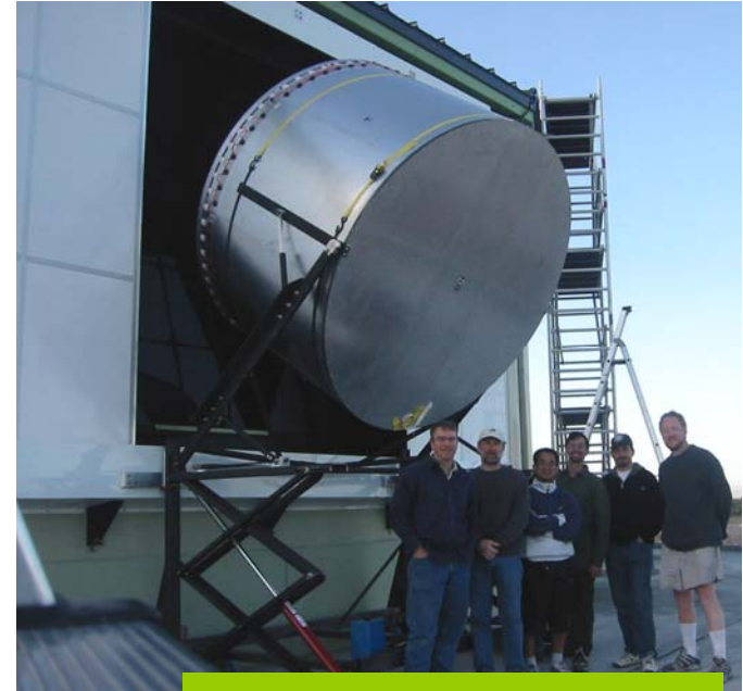
Drum for uniform camera illumination: end to end calibration
