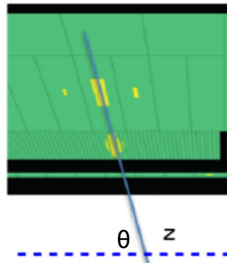
Measure  $\gamma$  direction with sampling calorimeter  $\rightarrow$  get Z of primary vertex
