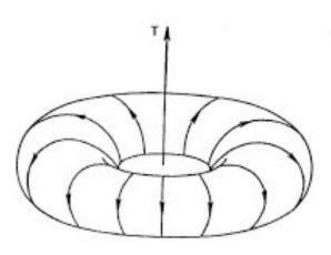
The simplest TDM model was given by Zel'dovich as a conventional solenoid rolled up in a torus and with only a poloidal current. For such stationary solenoid, without azimuthal components for the current or the electric field, there is only one magnetic azimuthal field different from zero inside the torus.
