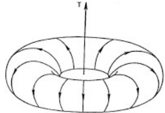
The simplest TDM model was given by Zel'dovich as a conventional solenoid rolled up in a torus and with only a poloidal current. For such stationary solenoid, without azimuthal components for the current or the electric field, there is only one magnetic azimuthal field different from zero inside the torus.
