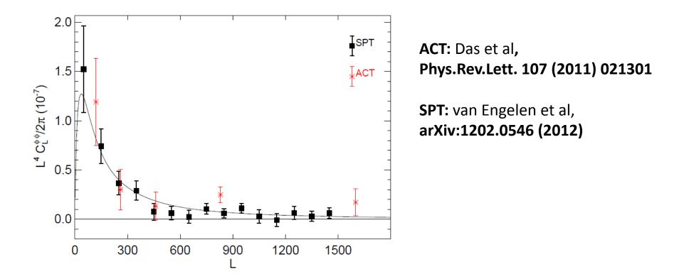
This non-gaussian signal has been measured by both ACT and SPT experiments, letting a reconstruction of the lensing potential.
