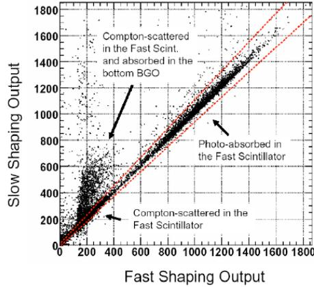
Figure 5: Results from the 50 keV run of the 2007 KEK beam test showing the correlation between events classified as ‘fast’ (horizontal axis) and ‘slow’ (vertical axis) by waveform sampling. Events between the two red lines correspond to clean hits in a fast scintillator and can be used to determine the beam polarisation.
