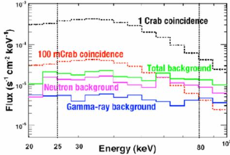
Figure 4: Valid and background event rates for PoGOLite: valid event rates expected from a 1000 mCrab source (black dotted line) and a 100 mCrab source (red dotted line) at a conservative  $4 \text{ g/cm}^2$  atmospheric overburden. The total (green solid line), neutron [9] (purple solid line) and gamma-ray [10] (blue solid line) backgrounds are shown. Neutrons and gamma-rays produced in the PoGOLite gondola structure by cosmic-ray particles have been calculated to be negligible.
