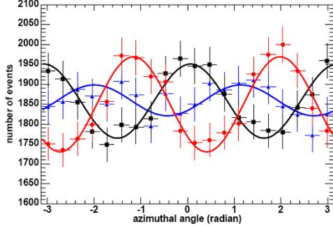
Figure 3: The polarization signal that PoGOLite will measure in 6 hrs at the top of the atmosphere for P1 of Crab Pulsar (defined in Figure 1) for the polar cap (red), slot gap/caustic (blue) and outer gap (black) models.
