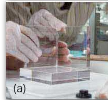
Well-type BGO active shield/collimator (0.5", 1" thick)
