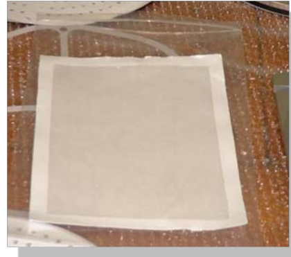
Collected filter • Glass fiber filter collection efficiency : 99.99% ( \phi 0.3 \mu\text{m} particle)
