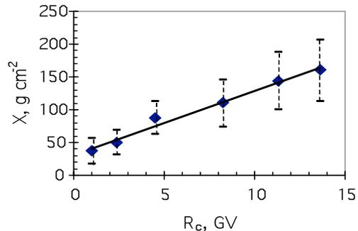
Figure 4: Atmospheric depth  $X$  corresponding to the maximum of muon flux in the atmosphere as a function of geomagnetic cutoff rigidity ( $R_c$ ) of location.
