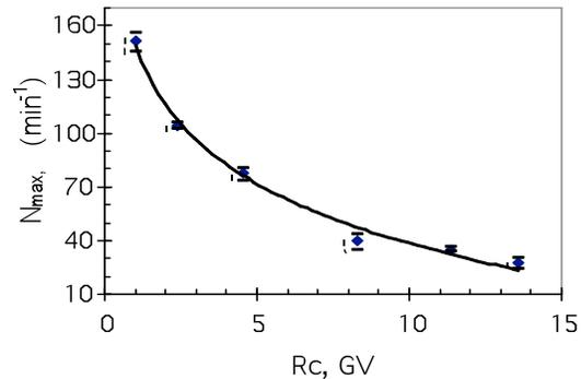
Figure 3: Maximum > 100 MeV muons count rate in the atmosphere as a function of the  $R_c$  of geomagnetic location.
