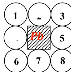
Figure 1: A detector scheme: eight Geiger counters (1-8) arranged as a vertical telescope, with a 2.5 cm thick *Pb* filter in the center.
