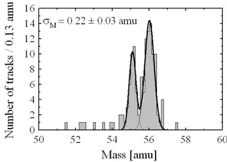
Figure 3: Mass distribution for iron nuclei in the CR-39 detector [6].
