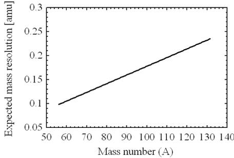
Figure 4: Variation of mass resolution expected for region  $56 \leq A \leq 132$  in the CR-39 detector [6].
