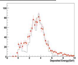
Figure 3: Deposited energy from events identified as oxygen using an SCD cut (7.5 < Z < 8.5) (red circles) and MC simulation results (histogram).
