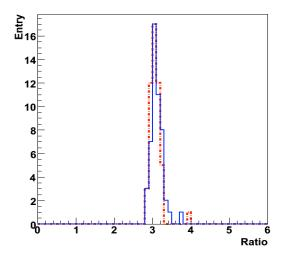
Figure 4: Ratio of signal sums between 50 and 150 GeV/c electrons before (blue solid line) and after (red dashed lihe) calibration for 50 different beam injection points. Uniformity of response improved from 4.8% to 3.8% after calibration.
