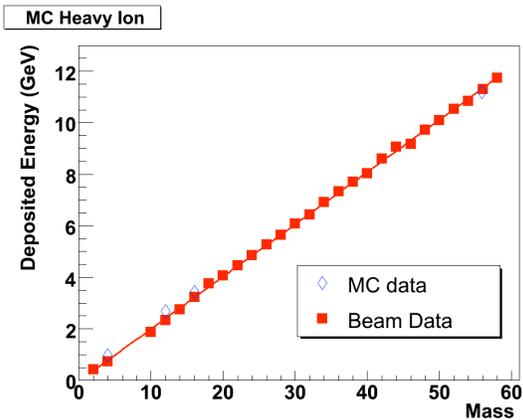
Figure 2: Energy deposit from  $A/Z = 2$  nuclear fragments produced by a 158 GeV/A indium beam incident on a thin target. Beam data (red triangles) after calibration are consistent with MC (blue circles) generated for  $Z = 2, 6, 8$  and 56.
