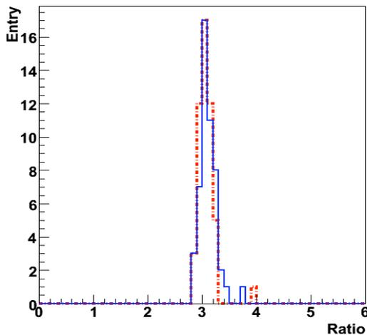
Figure 4: Ratio of signal sums between 50 and 150 GeV/c electrons before (blue solid line) and after (red dashed line) calibration for 50 different beam injection points. Uniformity of response improved from 4.8% to 3.8% after calibration.
