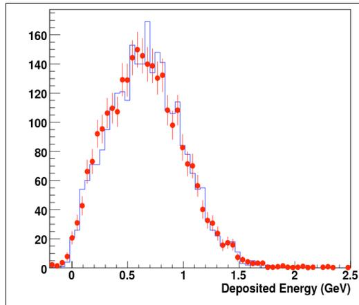
Figure 1: Deposited energy in 350 GeV/c proton beam (red circles) and MC events (histogram). Electronics noise and photon statistics were implemented in the MC. A cut on sum of deposited energy in several layers was applied to both beam and MC samples to select interacting particles.
