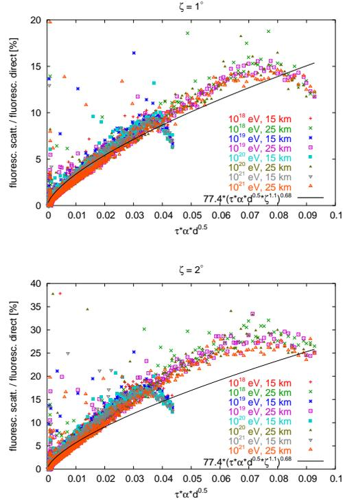
Figure 4: Comparison of fluorescence light scattering with results of [6] for  $\zeta = 1^\circ$  and  $\zeta = 2^\circ$ . The data points are results of this work, the lines represent the fit given in [6].
