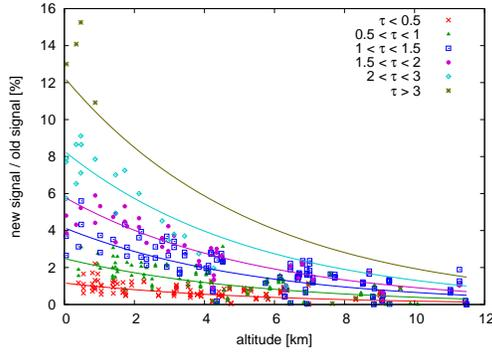
Figure 3: Contribution of multiple scattering for all values of the total horizontal attenuation length, in groups of the optical depth  $\tau$  along the shower-detector line of sight. The lines are fits of Eq.2 with mean values of the respective  $\tau$  intervals.
