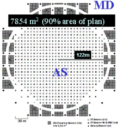
Figure 1: Schematic view of the Tibet-AS+MD array. Open squares and open circles represent the surface scintillation detectors that compose the Tibet-III AS array. Filled squares show the proposed Tibet MD array 2.5 m underground.
