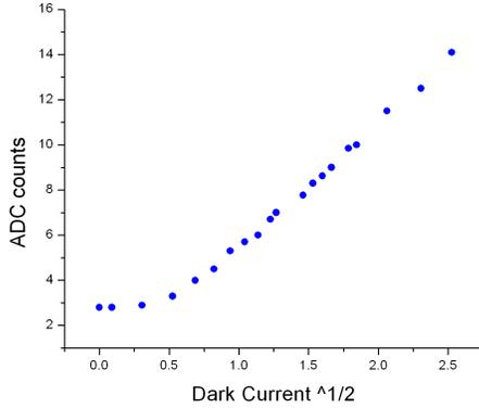
Figure 3: Pedestal RMS noise vs. SiPM dark current ( $\mu A$ ).
