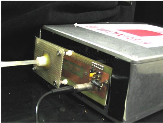
Figure 1: Laboratory test : one SiPM is optically coupled to a bundle of scintillating fibers.
