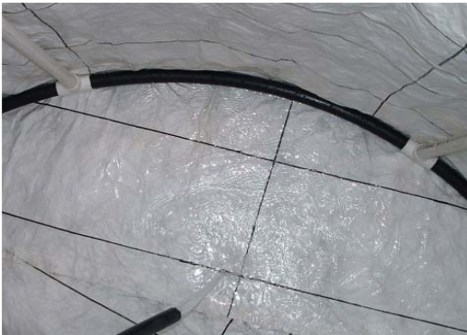
Figure 1: The water Cherenkov detectors consist of light-tight cylindrical containers of 4 m 2 cross section.
