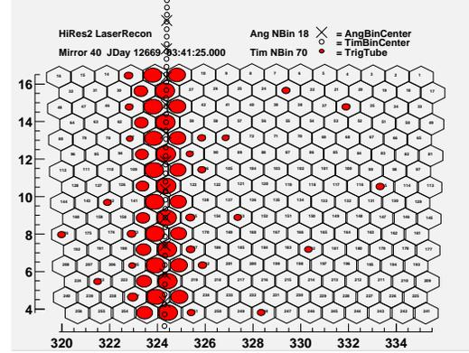
Figure 2: Typical vertical calibration laser shot as seen by HiRes2 from the night of 30 January 2003. Note that there are many more time bins than angular bins. Here angular bin centers are separated by  $1.5^\circ$ .
