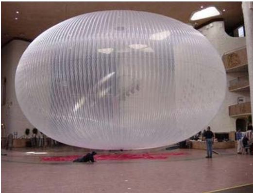
Figure 2: 14.3 m diameter, 200 gore model test balloon
