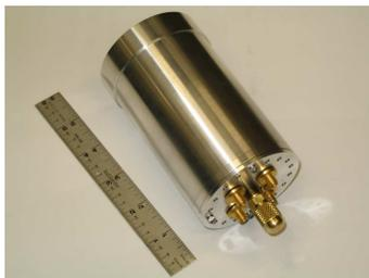
Figure 3: PMT enclosed with an aluminum hermetic case
