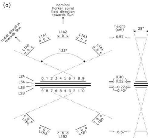
Figure 2: Schematic of the LET telescope
