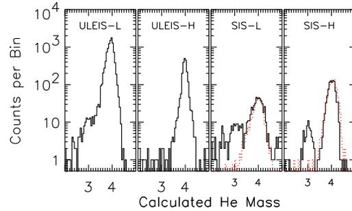
Figure 2: Helium mass histograms (solid lines) obtained by summing the data shown in Fig. 1. Dotted histograms shown for SIS-L and SIS-H illustrate distributions obtained from an event that had negligible  $^3\text{He}$ .
