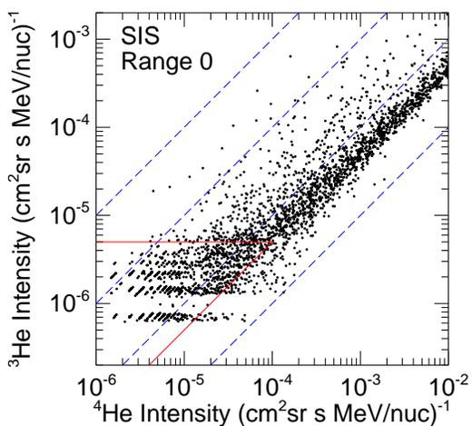
Figure 3: Distribution of daily average  ${}^3\text{He}$  and  ${}^4\text{He}$  from the lowest energy range measured in SIS. Dashed lines indicate  ${}^3\text{He}/{}^4\text{He}$  of 0.01, 0.1, 1, and 10. Days falling in the lower left region bounded by solid lines were selected as quiet days for this study.
