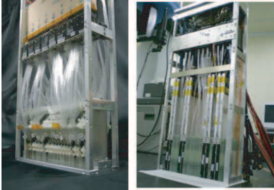
Figure 4: Left: the Arm#1 detector, which has been completed in July 2006. It has the tungsten plates with total length of 44 X_0 and 1.6 \lambda_I , 16 scintillator layers and 4 X-Y scifi layers at 6, 10, 30, 42 X_0 . Right: Arm#2 detector, which has been completed in April 2007. It has 4 X-Y microstrip silicon layers at 6, 12, 30, 42 X_0 instead of the scifi layers.
