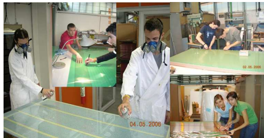
Figure 3: Students involved in the construction of their telescope MRPCs at the CERN laboratories.
