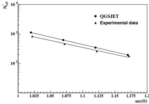
Figure 1: Acceptance corrected event numbers vs.  $\text{sec } \theta$  for the simulated and experimental data selected with the  $N_{\mu}$ - $N_e$  cuts. The fits with expression (1) providing the  $\lambda_{obs}$  values are also shown (continuous lines).
