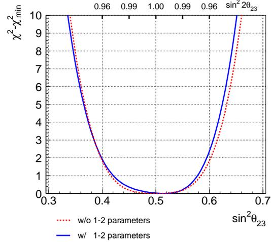
Figure 3: The  $\chi^2 - \chi_{\min}^2$  distribution as a function of  $\sin^2 \theta_{23}$  for oscillations without the 1–2 parameters (red dashed line) and with the 1–2 parameters (blue solid line) by the SK-I + SK-II atmospheric neutrino data.  $\theta_{13} = 0$  is assumed. For each  $\sin^2 \theta_{23}$  point, the other oscillation parameters are chosen to minimize  $\chi^2$ .
