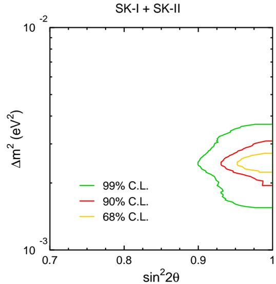
Figure 2: Allowed oscillation parameters for  $\nu_\mu \leftrightarrow \nu_\tau$  oscillations by the SK-I + SK-II data
