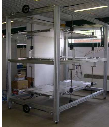
Figure 1: Typical set up of the MRPC telescope.
