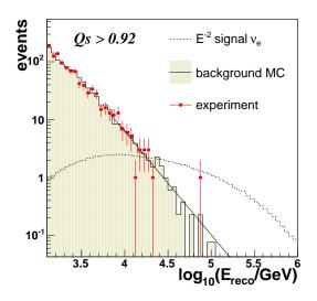
Figure 3: The reconstructed cascade energy distribution  $E_{\rm reco}$ . Shown are experimental data as well as background and signal Monte Carlo simulation after application of all quality cuts and a cut on the discriminating parameter Q > 0.92. The smooth line is a result of the power-law fit to the background simulation.
