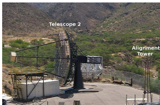
Figure 2: Purpose-built alignment towers have been constructed and placed at the “ 2f ” point for each telescope. In this image, the telescope is stowed (pointing north) and is not pointing at the tower.
