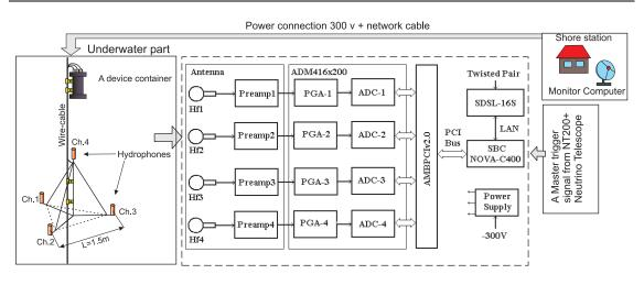
Figure 1: Schematic view of underwater 4-channel digital device for detection of acoustic signals from high energy neutrinos.
