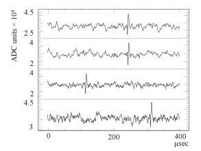
Figure 2: Sample of detected bipolar pulse.
