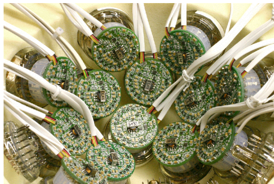
Figure 5: The high voltage end of the photomultiplier tubes fitted in the Styrofoam shell. Most of the attached cables are for testing purposes only.
