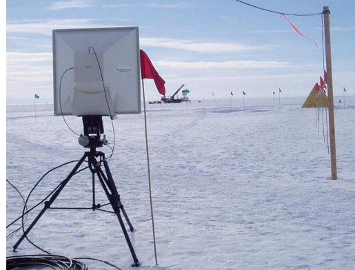
Figure 2: The ANITA ground pulser system. The surface horn antenna is in the foreground; the borehole discone antenna is \sim 20 m below the surface (under the yellow Scott tent). The ANITA payload is visible in the background, on the launch vehicle.
