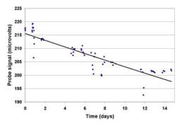
Figure 2: Trinity University measurement of relaxation time for charge on fused silica optic
