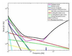
Figure 1: The theoretical charging noise contribution (solid green line) versus the total noise predicted for Advanced LIGO (solid black curve), assuming a total charge of  $10^{-11}$  coulombs and a relaxation time of  $4 \times 10^7$  s
