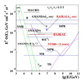
Figure 4: All-flavor neutrino flux predictions in different models of neutrino sources compared to experimental upper limits to  $E^{-2}$  fluxes obtained by this analysis and other experiments (see text). Also shown is the sensitivity expected for 3 live years of the new telescope NT200+.
