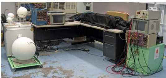
Figure 1: Experimental apparatus for measuring cosmic ray neutron spectra: (left) Bonner multi-sphere spectrometer; (right) scintillation counter.
