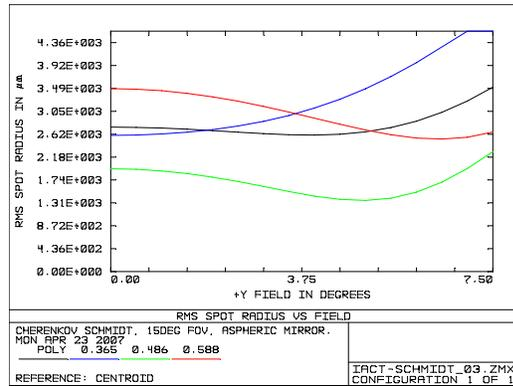
Figure 3: The monochromatic and polychromatic r.m.s. spot size as function of field angle. The vertical scale goes from (0 – 1)'.
