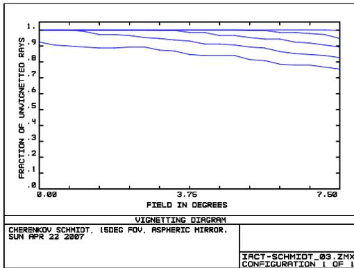
Figure 4: Vignetting as function of field angle for configurations with a 20m, 22m, 24m, 26m and 28m diameter mirror.
