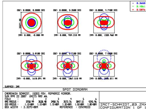
Figure 2: Spot diagrams for the 6 field positions between (0 - 7.5)° off-axis. The boxes are 5'.
