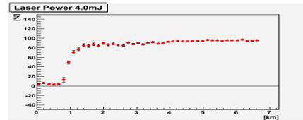
Figure 6: A sample of the correction factor for the PMT signal obtained using PMT and/or LED data for the laser energy 4mJ.
