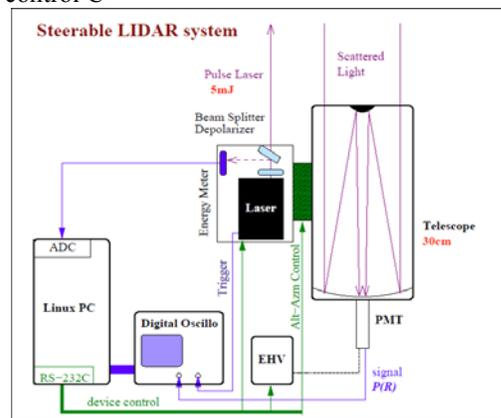
Figure 1: A block diagram of the LIDAR system.
