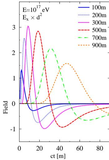
Figure 2: [color online] Electric field strength (multiplied by  $d^2$ ) at different distances from the shower core as function of time.
