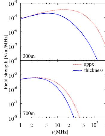
Figure 1: [color online] Frequency response of the pulse at 300 m and 700 m from the core for a  $10^{17}$  eV shower. In the calculations labeled 'appx' and 'thickness' the thickness of the pancake is zero (Eq. (16)) and 10 m respectively.
