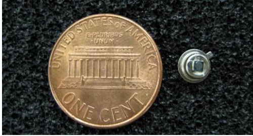
Figure 1: A 1 \times 1 \text{ mm}^2 active area Si-PM (a US one cent coin is shown for scale).
