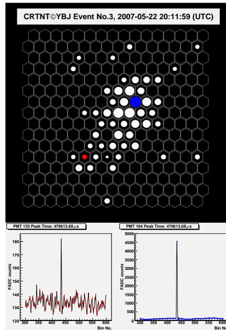
Figure 3: An example of CRTNT and ARGO-YBJ coincident event. Top panel shows the triggered pattern in PMT cluster. FADC histories of two firing tubes, marked with blue and red, are shown at bottom two panels
