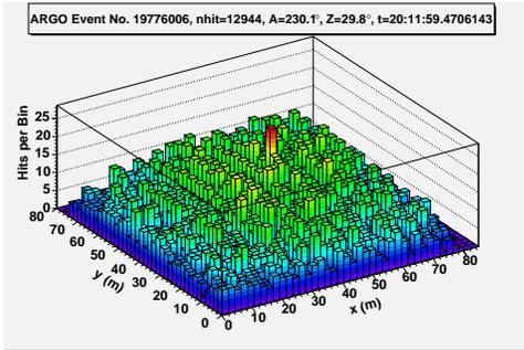
Figure 4: Hit map of the ARGO-YBJ carper array for the same event shown in Fig.3
