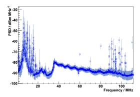
Figure 1: Spectral power density measured near the Balloon Launching Station using an LPDA and an Anritsu MS2711D spectrum analyser. The antenna signal was amplified using a low-noise amplifier [11] followed by an RG213 cable with a length of 160 m.
